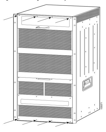
Figure 2 Installing the Panel Safety Cover
